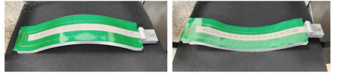
Fig. 1. Fabricated prototypes of the concave and convex standing-wave metasurface antennas: (a) Convex waveguide and (b) Concave waveguide.
