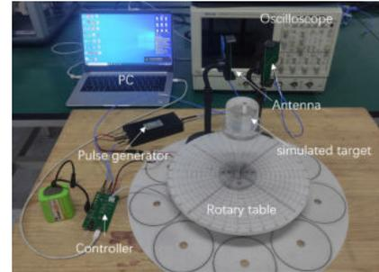
Fig. 1. The experimental time-domain microwave imaging system in our previous work.
