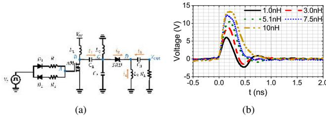
Fig. 3. (a) The circuit of the proposed sub-nanosecond pulse transmitter. The waveform of the fabricated sub-nanosecond pulse transmitter with (b) different value of  $L_3$ .
