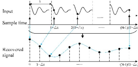
Fig. 4. equivalent time-sampling timing diagram.
