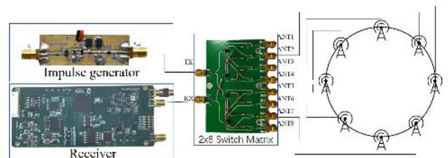
Fig. 2. Top-level block diagram of the real-time monitoring microwave ablation system.
