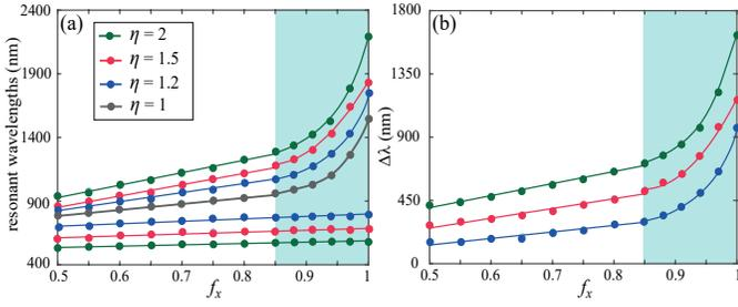
Fig. 2. The dependencies of (a) the resonant wavelengths  $\lambda_0$  (gray lines),  $\lambda_x$  (upper solid lines) and  $\lambda_y$  (lower dashed lines) and (b)  $\Delta\lambda$  on the  $f_x$  along the stretching direction for the fixed  $p$  and  $\eta$ .
