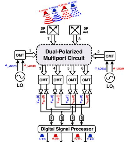
Fig. 1. Proposed dual-polarized metallic interferometric waveguide receiver systems.
