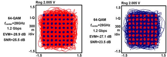
Fig. 2. Measured constellation diagrams of the proposed metallic interferometric waveguide receiver systems. (a) Vertical-polarization 64-QAM at 28 GHz. (b) Horizontal-polarization 64-QAM at 28 GHz.
