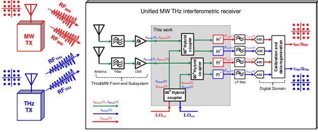
Fig. 3. Proposed unified microwave and terahertz interferometric receiver.
