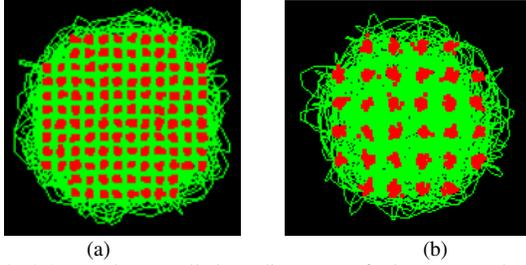
Fig. 4. Measured constellation diagrams of the proposed unified microwave and terahertz interferometric receiver. (a) 128-QAM at 5.8 GHz. (b) 32-QAM at 150 GHz.
