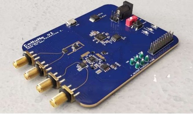
Figure 3 - Designed PCB comprising the measurement and processing chain of the system.
