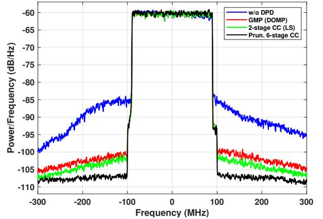
Fig. 3. Output spectra before and after DPD linearization considering different DPD models at near 600 coefficients.
