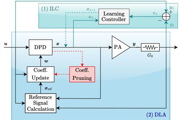
Fig. 1. Block diagram of the iterative learning control (1) and direct learning approach (2) including a model order reduction coefficient pruning block.
