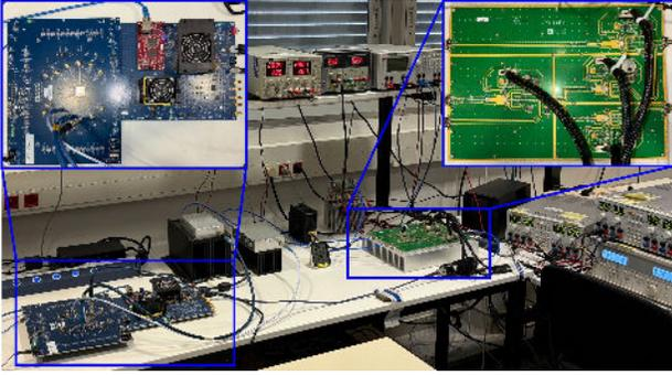
Fig. 2. Experimental setup including the transceiver board and the PD-LMBA.
