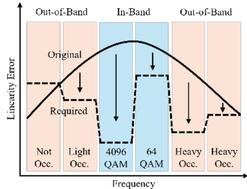
Fig. 1. Multimetric linearity requirements
