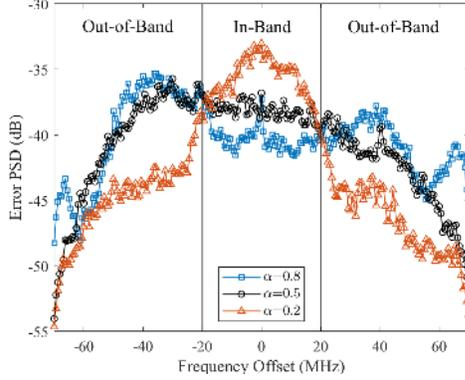
Fig. 3. Error PSD comparison at the same NMSE threshold.
