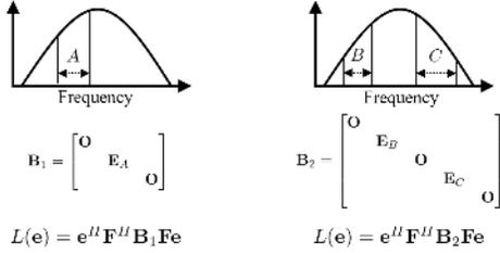
Fig. 2. Distinguishing the linearity error in different frequency regions.
