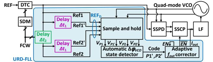
Fig. 1. Architecture of the proposed fractional-N sub-sampling PLL with URD-FLL.
