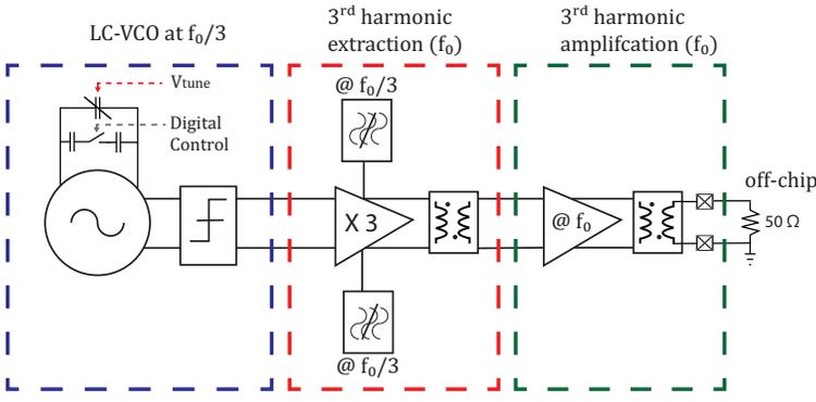
Fig. 1. Block diagram of the 60 GHz frequency generator
