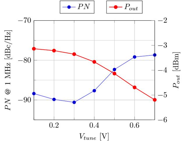
Fig. 3. Phase noise and output power behaviour against the tuning voltage
