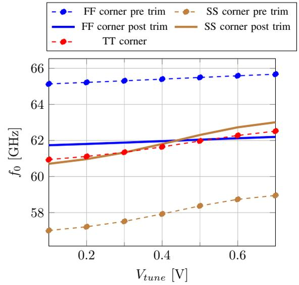
Fig. 2. Frequency generator's response over process variations before and after trimming
