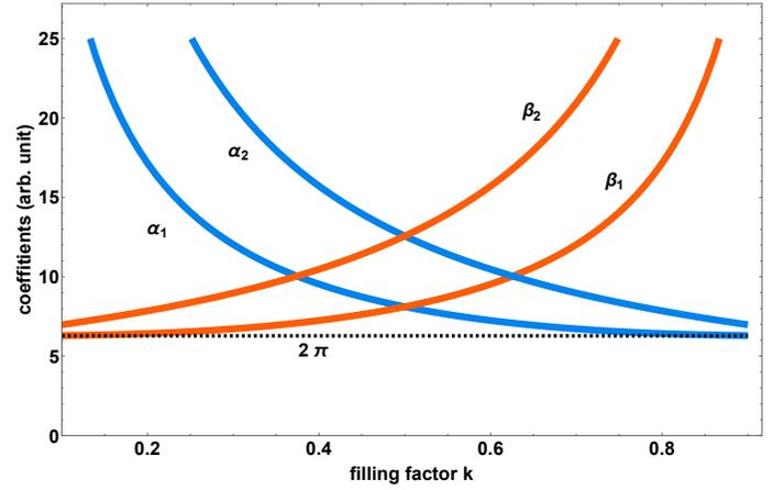
Fig. 2. Filling factor  $k = L_2/(L_1 + L_2)$  dependence of first solutions  $\alpha_{1,2}$  and  $\beta_{1,2}$  coefficients corresponding to the first frequency branch.
