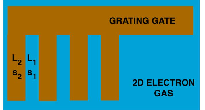
Fig. 1. Sketch of grating-gate FET with alternating two types of regions – ungated (length  $L_1$  and plasmonic velocity  $s_1$ ) and gated (length  $L_2$  and plasmonic velocity  $s_2$ ).
