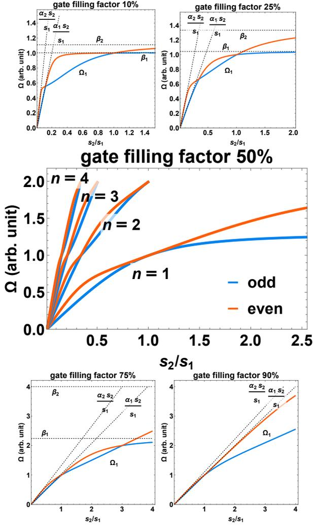
Fig. 3. First frequency branch  $\Omega = \omega s_1 / (L_1 + L_2)$  depending on normalized plasma wave velocity  $s_2/s_1$  for different values of filling factor  $L_2 / (L_1 + L_2)$
