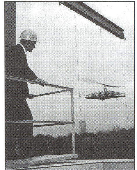
Bill watches the helicopter in flight. Stabilization wires pass through the center of the helicopter and through the ends of two outrigger rods. The demonstration lasted 10 hours with the helicopter hovering at an altitude of 60 ft.
