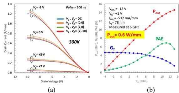
Fig. 3. (a) Pulsed I-V and (b) power-sweep characteristics of a p-type GaN/AlN HEMT on an AlN free-standing substrate.
