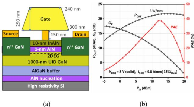
Fig. 2. (a) Cross-section schematics and (b) power-sweep characteristics of an InAlN/GaN HEMT on a Si substrate.
