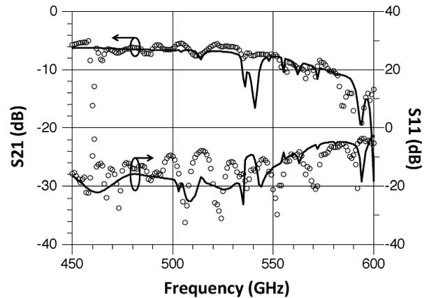
Fig. 4. Measured S-Parameters of “through” structure to validate WR 2.2 dipole transition. Note that solid lines indicate simulated performance and circles indicate measured performance.
