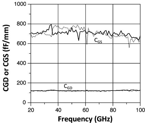
Fig. 2. Two extractions of  $C_{GS}$  and  $C_{GD}$  with successive calibration and measurements.
