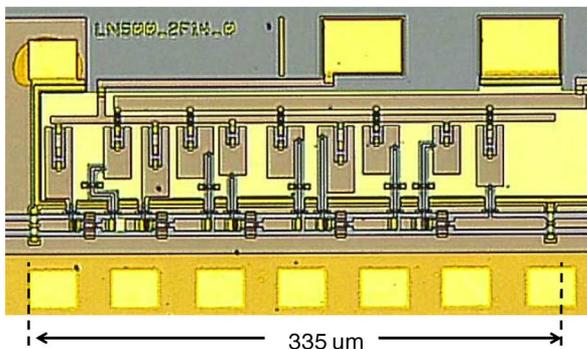
Fig. 3. Microphotograph of amplifier portion of chip.
