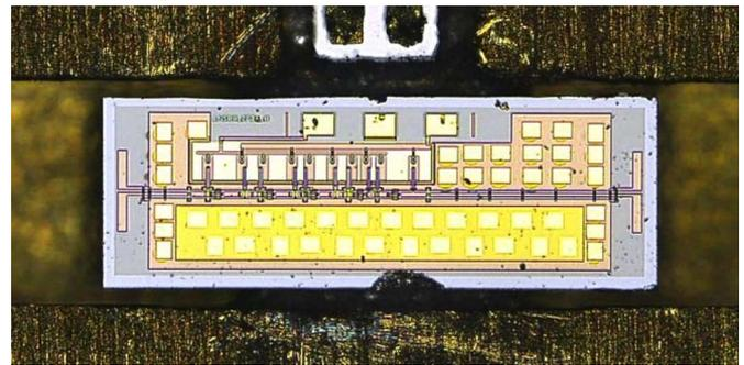
Fig. 1. Microphotograph of 480 GHz LNA in split block housing. The signal is electromagnetically coupled to the chip by monolithically integrated dipole probes.
