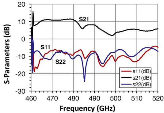
Fig. 5. Measured S-Parameters of amplifier module.
