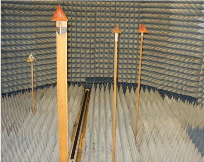
Fig. 20. Measurement setup used for moving target measurements. The photograph was taken at the beginning of the target movement and shows the case where three CCs are static, whereas one is mounted on a rail and moving.
