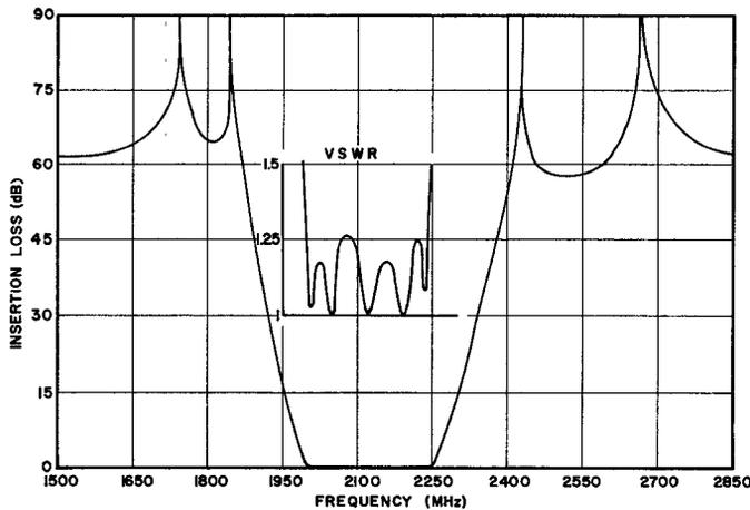
Fig. 8. Insertion loss and VSWR characteristics of experimental filter.
