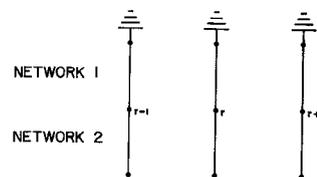
Fig. 3. The coupled-line realization of the basic resonated section.
