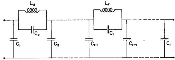
Fig. 1. The odd-order low-pass prototype elliptic function filters.
