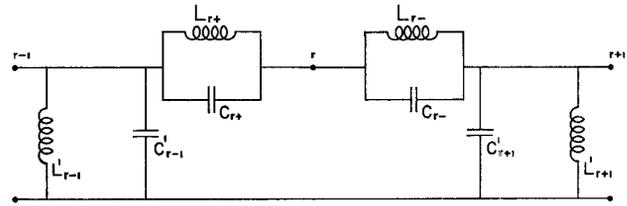
Fig. 2. A typical resonated pi section.
