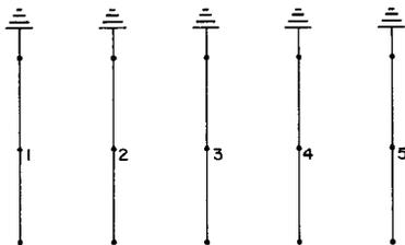
Fig. 4. Degenerate realization of a two-section filter.
