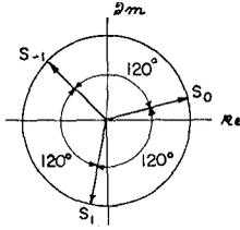
Fig. 5—Scattering matrix eigenvalues for a 3-port circulator.
