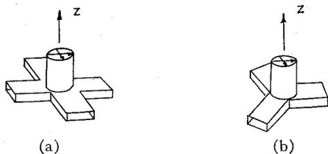
Fig. 2—(a) Four-arm turnstile junction.
