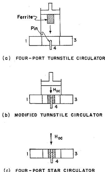
Fig. 3—Modifications of the 4-port turnstile junction.
